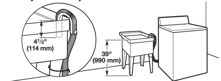
Minimum capacity: 20 gal. (76 L). Top of laundry tub must be at least 39" (990 mm) above floor; install no higher than 96" (2.44 m) from bottom of washer.
