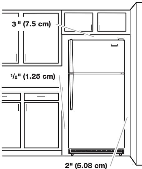
To ensure proper ventilation for your refrigerator, allow for a 1/2" (1.25 cm) space on each side. Allow 3" (7.5 cm) of space between overhead cabinets and refrigerator top. Allow at least 1" (25.40 mm) between back of cabinet and the wall. If your refrigerator has an ice maker, make sure you leave some extra space at the back for the water line connections.
