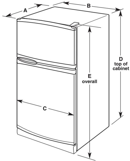
Dimensions "D" and "E" include rollers extended 3/4" (1.9 cm)
