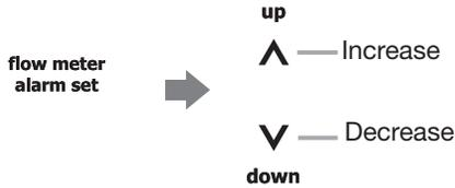
Choose the flow meter alarm setting from the following options: 10 - 60 gallon (40 - 240L) (In 5 gallon (20L) intervals), 70 gallon (260L), 80 gallon (300L), 90 gallon (340L), 100 gallon (380L) , 990 gallon.
