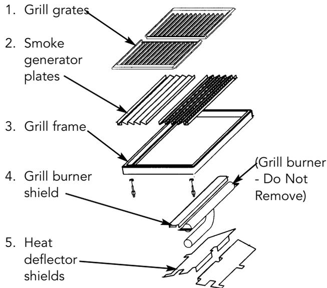
Clean greasy parts with a household grease solvent such as household ammonia and water. If necessary, a soap filled steel wool pad can be used on the grill frame shield, grill burner, and grill heat deflector.
