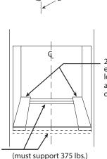
2 x 4 or equivalent runners level with bottom of cutout and flush with sides of cutout or solid bottom floor.
