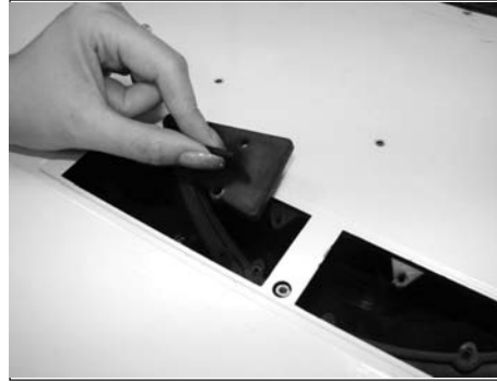
6. Remove (2) interior recirculating panels.
