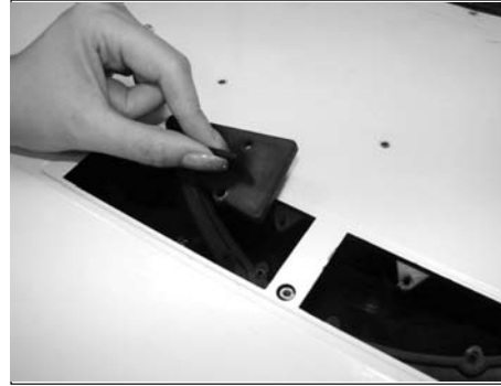
6. Remove (2) interior recirculating panels.
