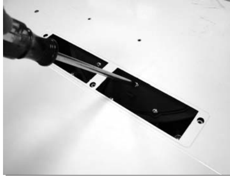
5. Remove each of the 5 screws holding the (2) interior recirculating panels.
