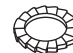
1 safety screw and lock washer, to secure the blower: (screw is marked with red or blue paint)
