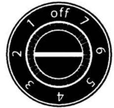
To start your wine cellar, use a screwdriver to turn the control clockwise to the middle thermostat setting. Once the wine cellar is loaded allow at least 48 hours for the unit to stabilize before making any adjustments to the initial setting.
