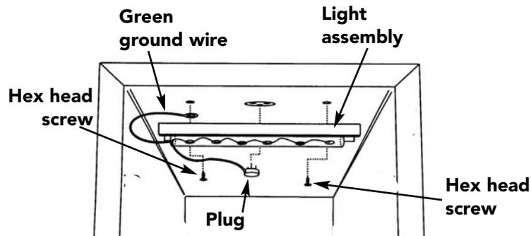
To install the new light assembly, screw in the green ground wire screw and the screw located on the right with a 5/16" hex head screwdriver and plug the light unit in.
