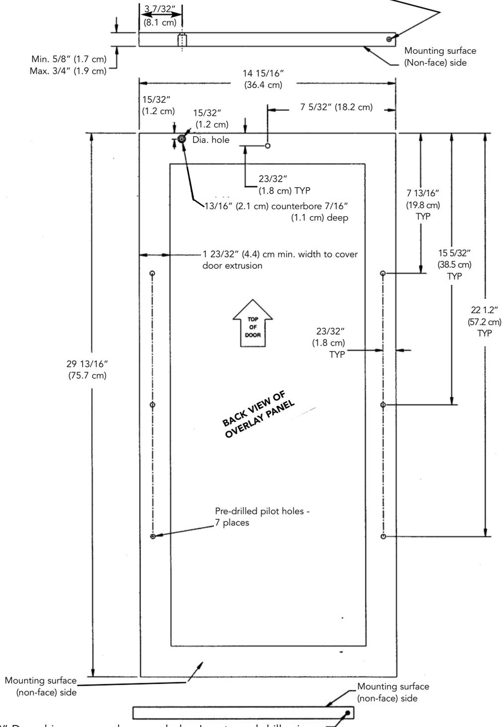
1/4" X 3/8" Deep hinge screw clearance hole. Locate and drill using door hinge hole after the door has been aligned to the unit and when the wood is positioned on door
