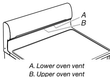
The oven vents release hot air and moisture from the ovens, and should not be blocked or covered. Blocking or covering the vents will cause poor air circulation, affecting cooking and cleaning results. Do not set plastics, paper or other items that could melt or burn near the oven vents.
