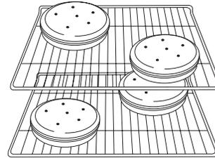
If oven has been converted for use with LP gas, use rack positions 3 and 5. Place cakes on racks as shown in the previous illustration.
