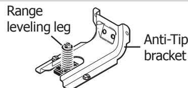
To check if the anti-tip bracket is installed properly, use both arms and grasp the rear edge of range back. Carefully attempt to tilt range forward. When properly installed, the range should not tilt forward.
