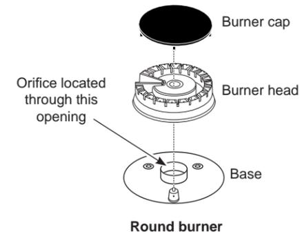
B. Using a 7 mm or 9/32" nut driver, remove the top burner orifices. These may be accessed through the burner opening in the base.
