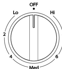
The control knobs can be set to anywhere between HIGH and LOW. Push in and turn to setting.
