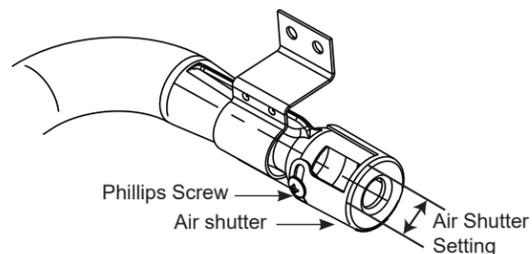
With a Phillips head screwdriver, loosen the screws securing the air shutters on the burners and adjust the air shutters according to chart above.
