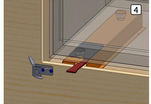
**L**astly, take the EuroTrim™ and click it into position. If you are satisfied with the installation, remove it one more time, peel off the protective PVC coating from the EuroTrim™ and click it into place for its final mount. (5)
