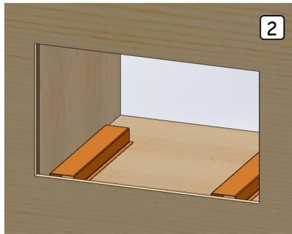
**P**lug in the microwave and place it on the runners. Center the microwave within the opening. Temporarily mount the EuroTrim™ and mark the location of its outside corners with a non-permanent marker or pen. Bend the magnet mounts as shown and screw them onto the front of the panel. Keep about 1/4"-inch (6mm) distance from the marked outside corners. Bend the flaps
