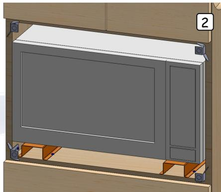
Then, take the EuroTrim™ and click it onto the magnet mounts. Next, open the microwave door and check for proper clearances. Adjust the alignment of the EuroTrim™ by removing it briefly and repositioning the flaps of the magnet mounts.
