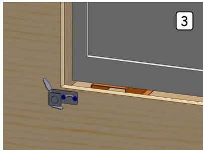
of the magnet mount as required to fine-tune the alignment between the EuroTrim™ and the microwave. Next, open the microwave door and check for proper clearances. Adjust the alignment of the EuroTrim™ by removing it briefly and repositioning the flaps of the magnet mount until you are satisfied. (3)
