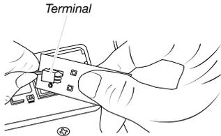
5. Replace a new LED, and snap it into the hook.
