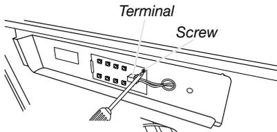
4. Replace a new LED, fasten the screw back.
