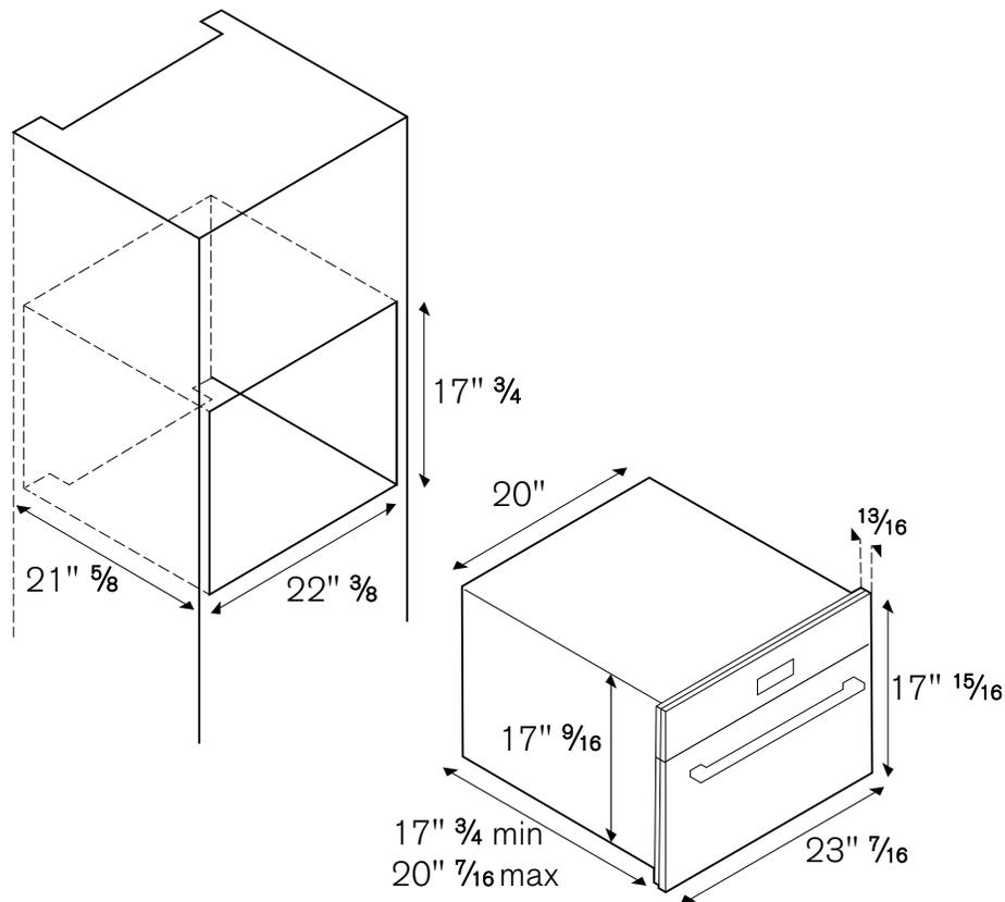
The minimum gap between the kitchen cabinet upper or lower panel and the appliance is  $\frac{1}{8}$ ". This dimension must be added to the height listed in the drawings.
