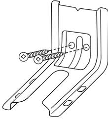
5. Using the Phillips screwdriver, mount anti-tip bracket to the wall or floor with the two #12 x 1 $\frac{5}{8}$ " screws provided.
