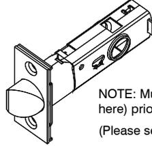
NOTE: Must attach faceplate to latch (as shown here) prior to installing latch in door.
